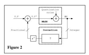
The input command can only change once per reference cycle, whilst the ideal correction transient is much shorter. In fact, the distortion associated with any PFD output pulse cannot be dealt with until one whole cycle later.
