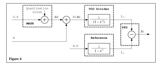
VCO frequency and period of a fractional-N synthesizer are related to reference period by:
