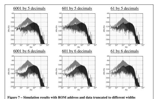
All loop components, including the VCO, were simulated as perfect and noiseless. The only noise sources were: PWM distortion; MASH quantization; and the finite numerical precision of the simulator.
